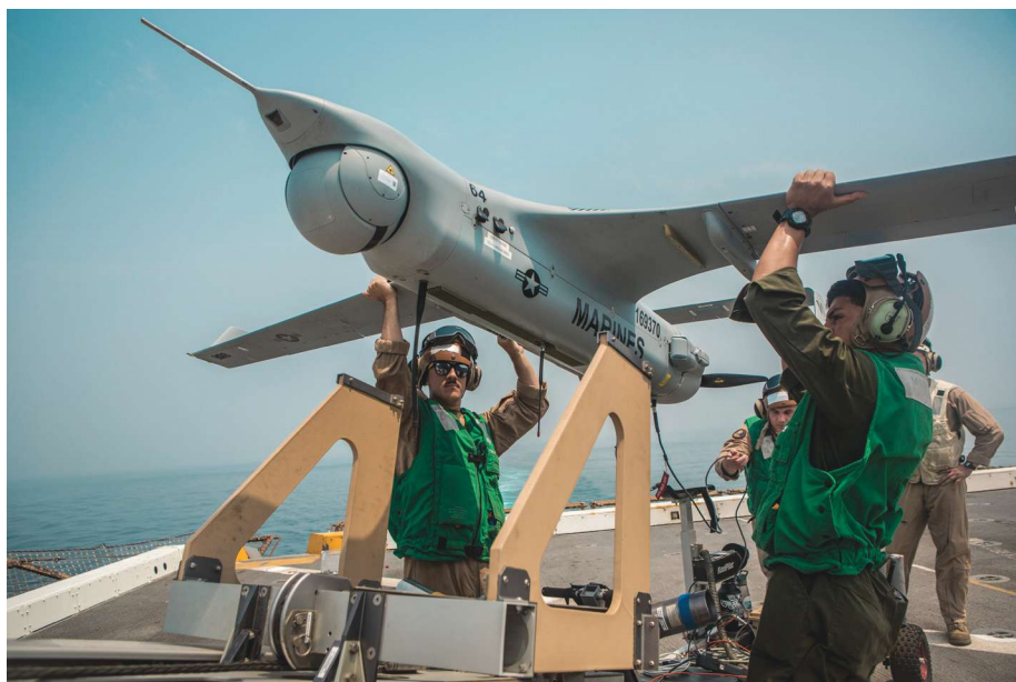
Marines with Marine Medium Tiltrotor Squadron 163 (Reinforced), 11th MEU lift an RQ-21A Blackjack UAS onto a launcher before flight operations aboard the amphibious transport dock ship USS John P. Murtha (LPD 26). (Photo by Adam Dublinske.)
