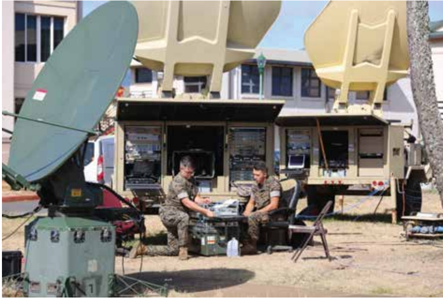
LCpl William Coward (left), a digital wideband technician, and LCpl Robert Murphy, a satellite operator, both of 3rd Marine Regiment, test a very small aperture terminal satellite system during ISLAND MARAUDER 21 on 9 August at Marine Corps Base Hawaii. ISLAND MARAUDER is an annual, Marine Corps Systems Command-led exercise enabling Marines to assess and familiarize themselves with communications gear. This year's exercise was nested under the Navy's LARGE SCALE Exercise 21. (Photo by Samantha Bates.)
