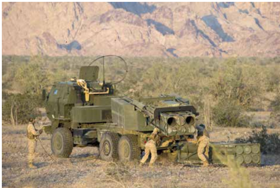
M142 High Mobility Rocket System could provide Marine “stand-in” forces with the range and lethality needed to contribute to a naval campaign. (Photo by Cpl Aaron James Vinculado.)
