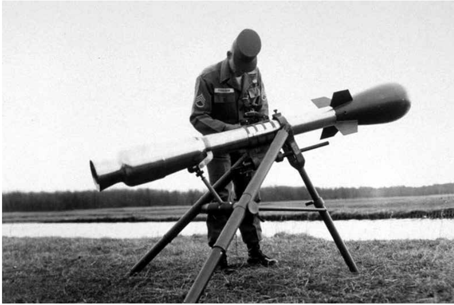
The “Pentomic Era” saw U.S. Army development of tactical nuclear weapons systems like the M28/29 “Davy Crockett” recoilless gun with M-388 sub-kiloton fission warhead to arm novel infantry formations. (U.S. Government DOD/DOE photograph.)
