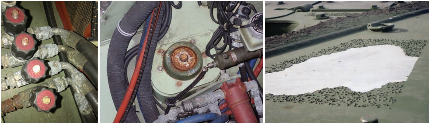
Figure 1. Corroded hydraulic control unit fittings, suspension strut mount, and delaminated exterior paint coating exposing a bare metal substrate. (Figure provided by Eric Brown.)
