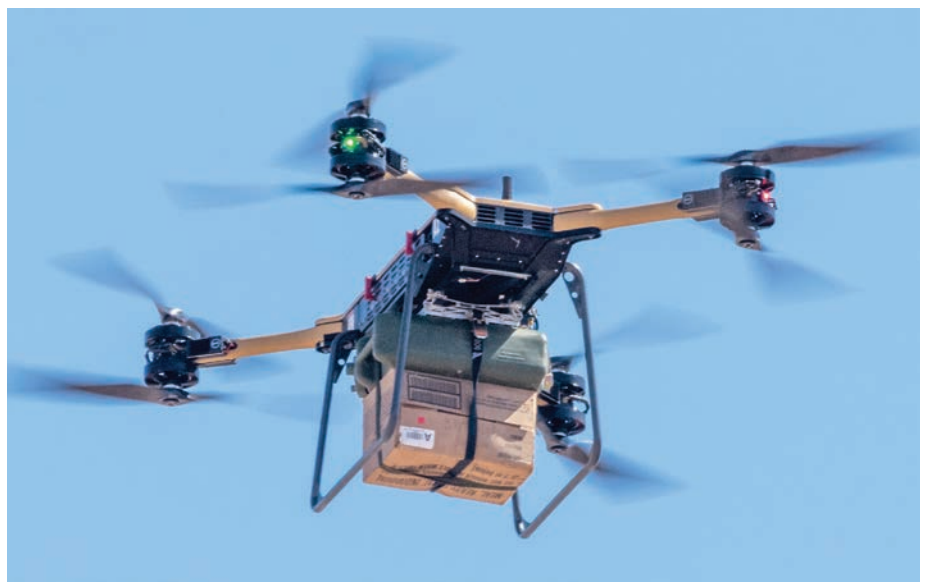
Future transformational resupply capability, Unmanned Logistics System-Air, undergoing operational testing by MCOTEA at Yuma Proving Grounds, Yuma, AZ. (Source: MCOTEA.)
