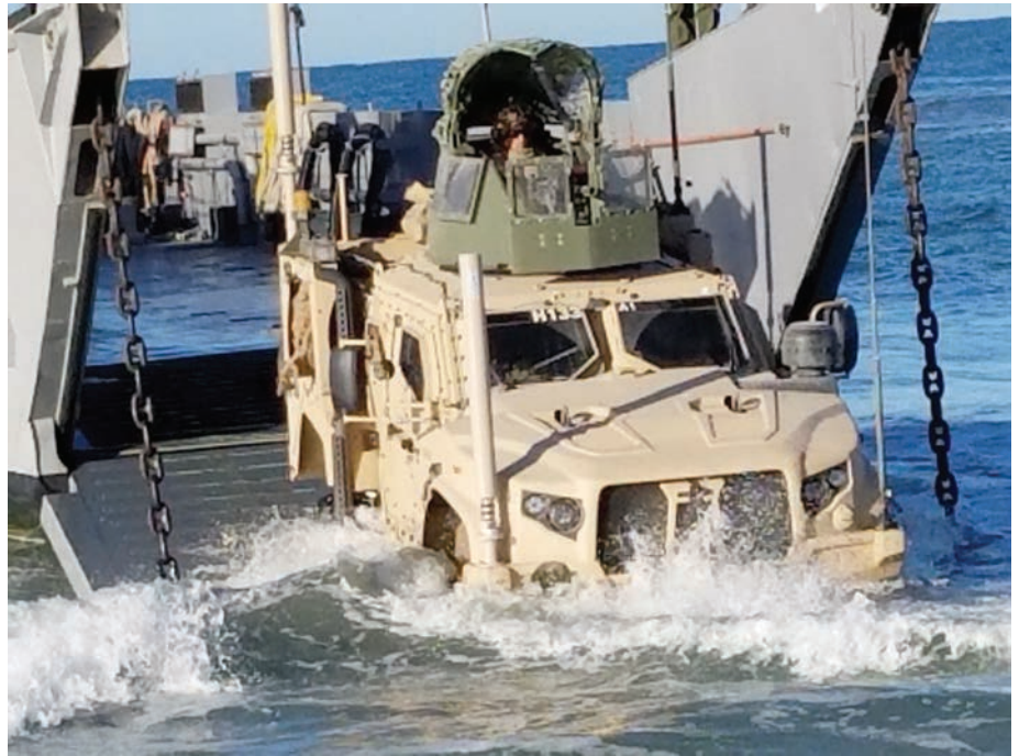
Joint Light Tactical Vehicle debarking from Landing Craft Utility boat to demonstrate transportability during operational test at Camp Pendleton, CA. (Source: MCOTEA.)
