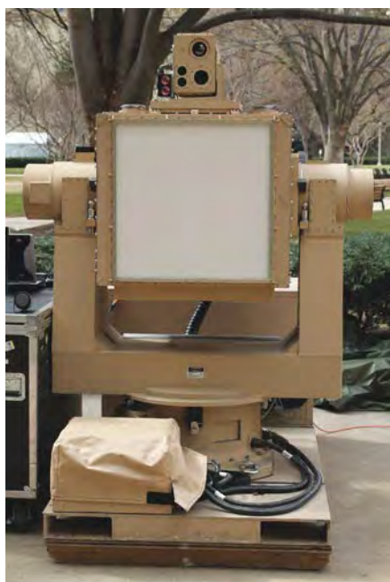
Solid-state active denial technology is a smaller, next-generation active denial system that will use directed energy to stop, deter, and turn back advancing adversaries. (Photo by Jamal B. Beck, JNLWD.)
