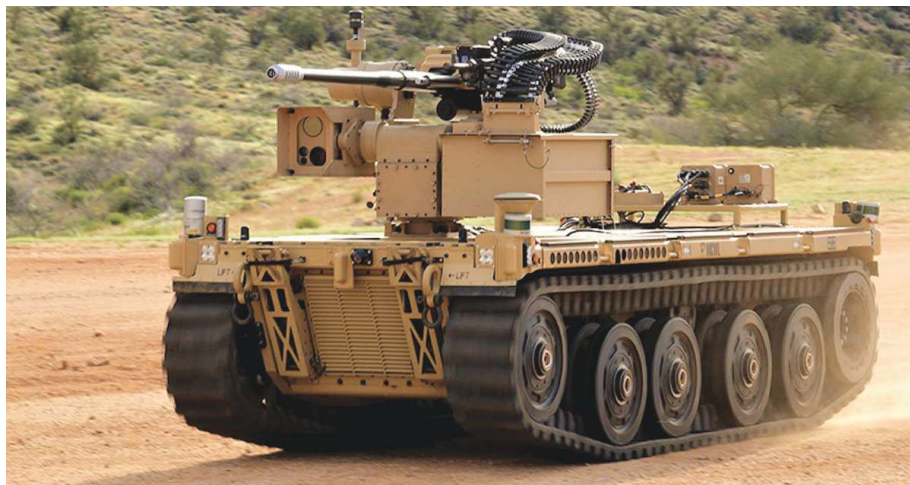
Figure 3. The EMAV is an unmanned ground vehicle developed by the MCWL, designed to host both commercial and government-owned MMPs. (U.S. Marine Corps photo.)
