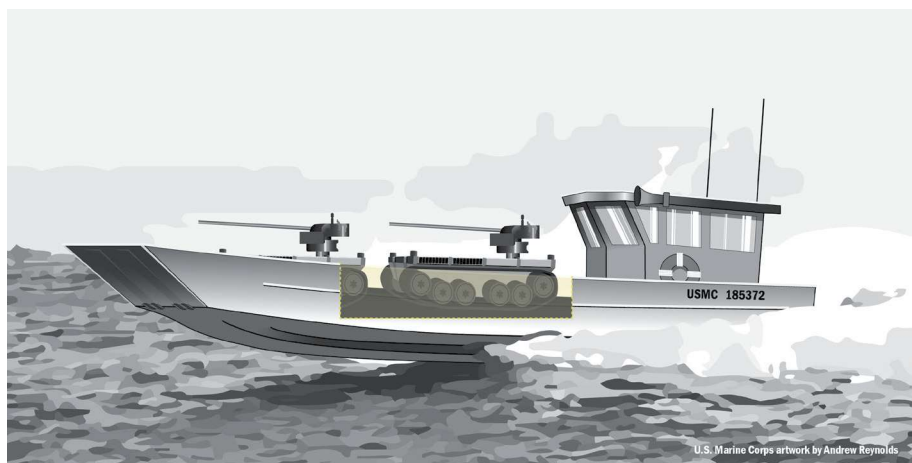
Figure 1. Artistic rendering of a Small High-Speed Amphibious Role-Variant Craft (SHARC) carrying two Expeditionary Modular Autonomous Vehicles (EMAV). (Image by Andrew Reynolds.)
