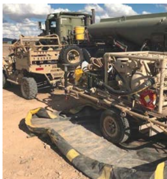
47 Cover Article The Marine Corps tactical air-ground refueling system. (Marine Corps photo.)
