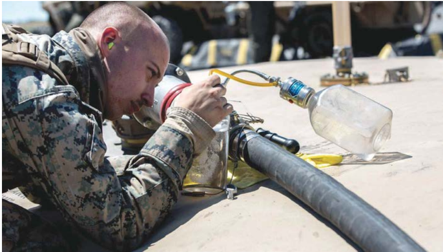
A bulk fuel specialist extracts fuel using an aviation test kit. DLA-provided fuel is one of the Service's high demand items. (Photo by LCpl Juan Anaya.)
