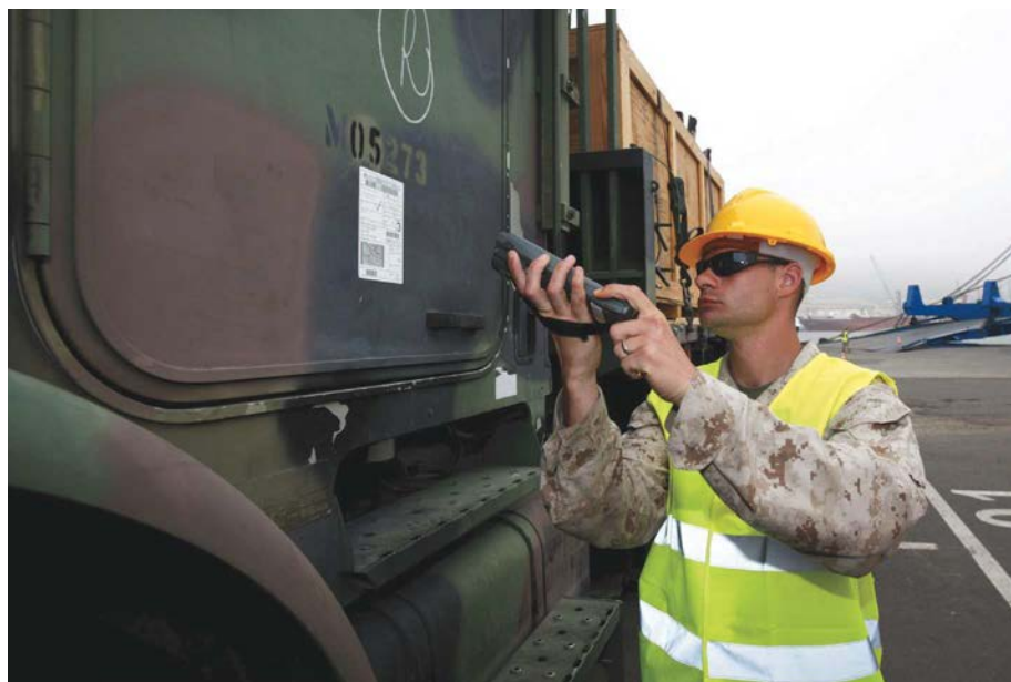
The vehicle is being tracked using a radio frequency identification tag. (Photo by LCpl Lydia Davey.)
