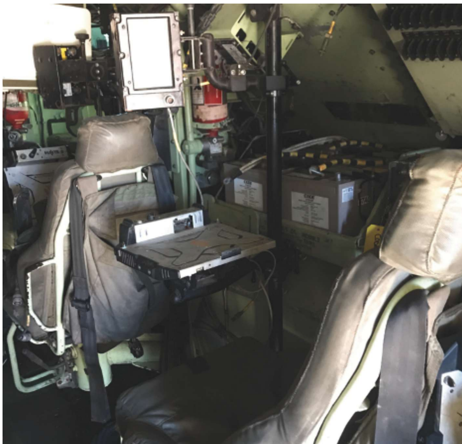
Photo of the back of a C7. One of six workstations in the AAVC7. Each workstation can choose to listen to, talk on, or ignore the six VHF nets, HF net, SatCom net, UHF-line of sight net, and Iridium satellite phone connection over headphones connected to the screen at the top of the image. A networked ruggedized laptop can be placed in the mount at the middle of the image.
