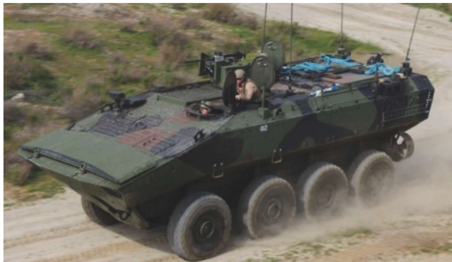
The ACV-C will share a common hull with the ACV-P, with twice the number of VHF antennas, as well as an HF antenna, and one satellite communications antenna.
