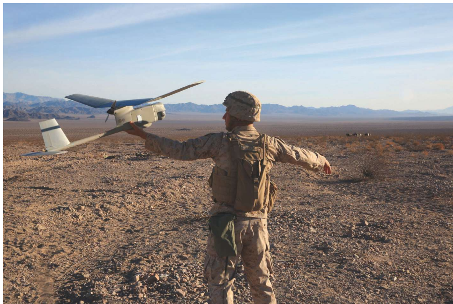
The LCE has Group 1 UASs like the RQ-11B Raven. (Photo by LCpl Austin Mealy)
