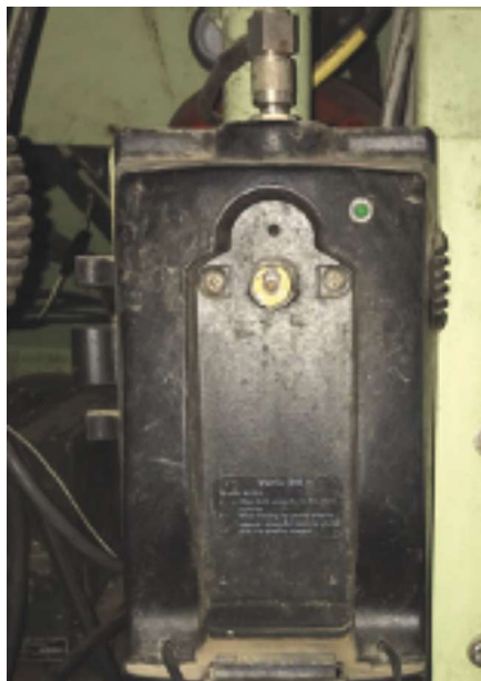
The AAVC7's mount for an Iridium phone. This antiquated mount, which does not work with the current Iridium phones, stops a battalion staff from using the Iridium on-the-move.
