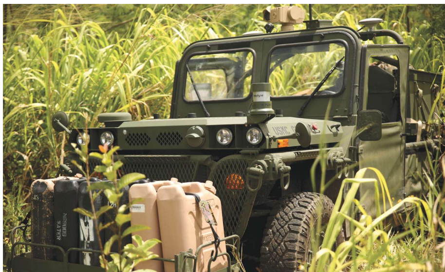
The Ground Unmanned Support System (GUSS) showed that a UGV did not need to be “remote controlled” by a dedicated Marine. (Photo: Courtesy MCWL.)
