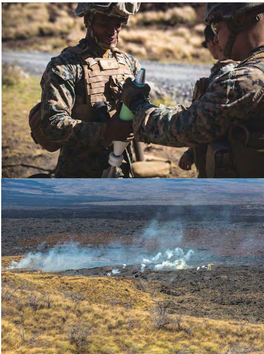
The 81mm flash-bang munition integrates flash-bang counter-personnel technology with existing 81mm mortar systems to suppress, move, and/or deny personnel access to or from an area. (Photos by LCpl Adam Montero.)
