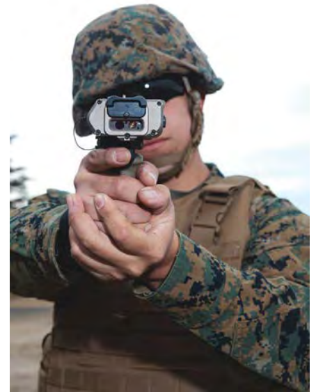
The ocular interruption system is a light emitting, non-damaging, eye-safe device fielded to warn and suppress individuals at a 10-500 meter standoff. (Left photo courtesy JNLWD; right photo by Mimi Ho, JNLWD.)
