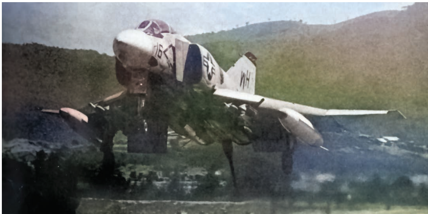
A Phantom II returned to its home base at Chu Lai after completing a mission. Its tailhook was used to catch an arresting cable, much the same way a plane lands aboard an aircraft carrier.
