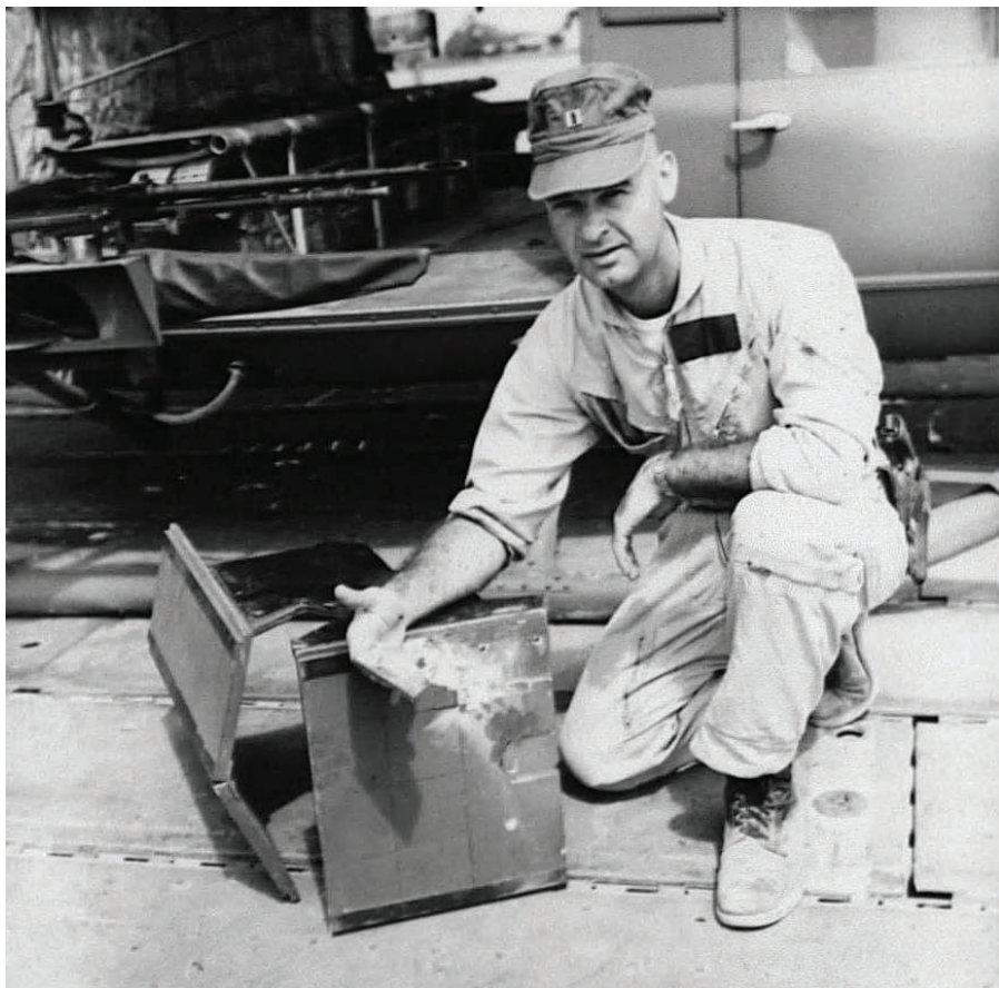
In April 1966, Capt William Huffcut of VMO-6 shows the armor plate surrounding his seat, which stopped a .50-caliber round.
