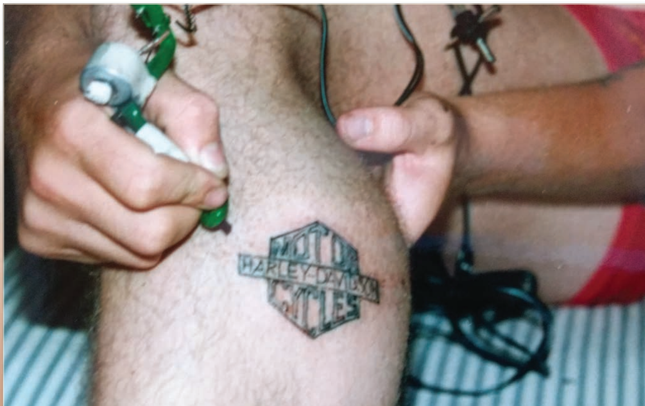
Eric Althen’s homemade tattoo machine. The motor extracted from a cassette player is mounted to the top of a toothbrush. When powered up, it rapidly feeds a length of guitar string through the hollow tube of an old Bic pen ink reservoir.
