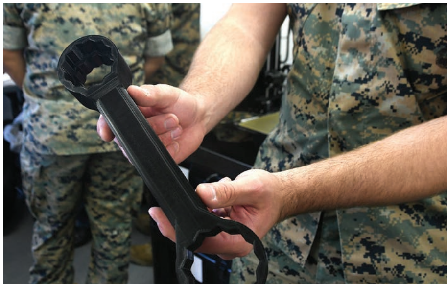
A Marine holds a 3D-printed universal load stud wrench at MCTSSA Camp Pendleton, Calif., April 27. Earlier in the month, a team tested and evaluated the XFAB, a portable additive manufacturing lab that once fielded to the fleet will give Marines the ability to fabricate replacement and repair parts in an expeditionary environment.
