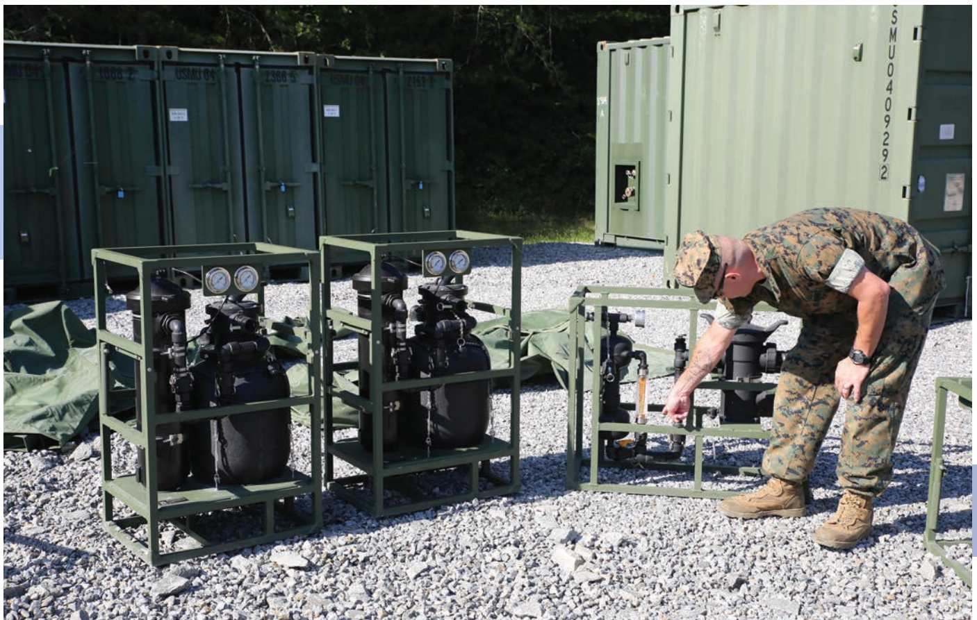
MSgt Ryan Miller, project officer for Family of Water Systems at Marine Corps Systems Command, assembles the Lightweight Water Purification System with the new Enhanced Production Module. (Photo by Kaitlin Kelly)
