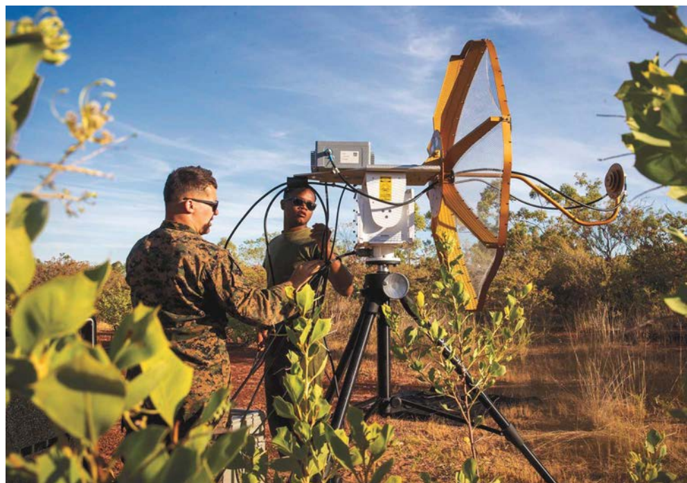
LCpl Brayden Broens and LCpl Dominick Rollan with MRF-D set up the ground data terminal at an RQ-21A spoke site in Bradshaw Field Training Area, Northern Territory, Australia, Aug. 9. (Photo by Cpl Harrison Rakhshani, USMC)
