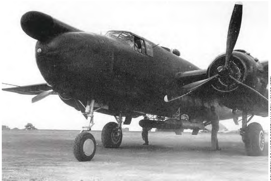
VMB-612's PBJs stood out in daylight photographs due to their midnight-blue paint scheme. Note the two Tiny-Tim rockets loaded on the belly racks.
