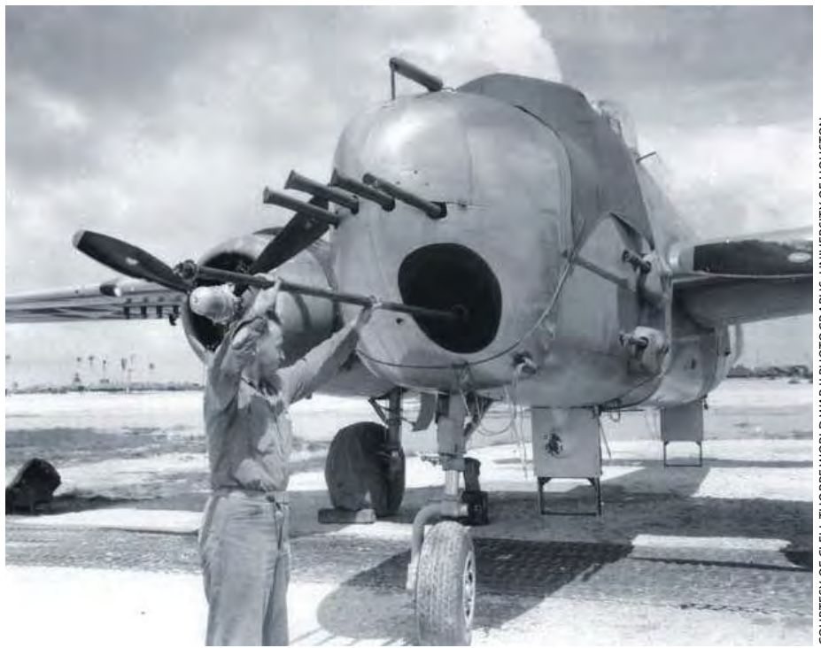
MTSgt Lloyd Staggs of VMB-613 cleans a PBJ-1H's 75 mm cannon. Above his head are four .50-cal. machine guns, and rocket racks can be seen under the wings.
