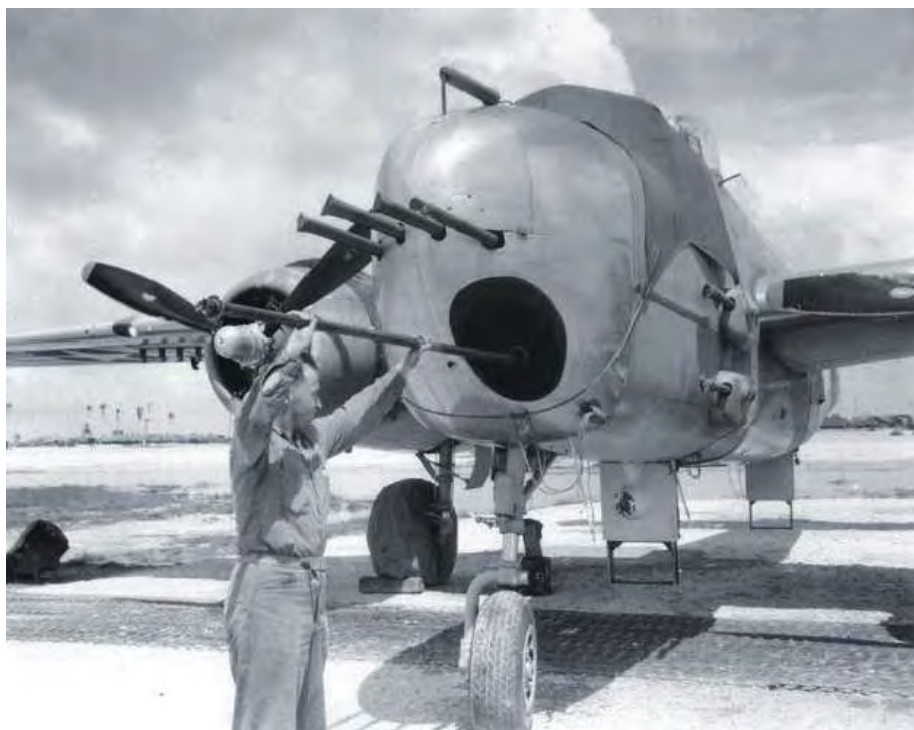
MTSgt Lloyd Staggs of VMB-613 cleans a PBJ-1H's 75 mm cannon. Above his head are four .50-cal. machine guns, and rocket racks can be seen under the wings.
