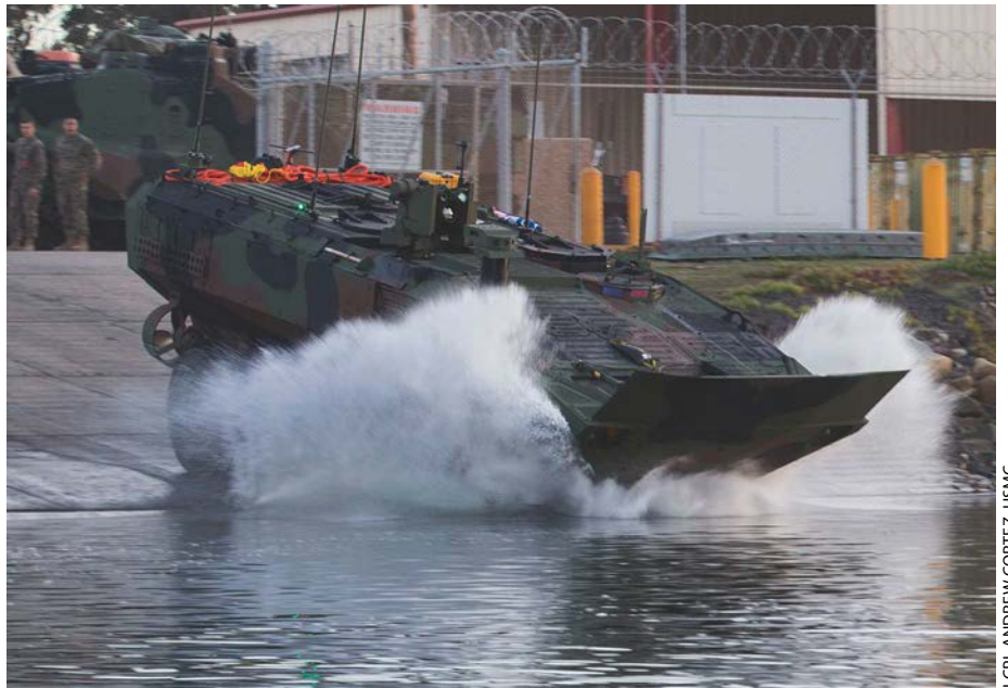
Marines with AVTB, Marine Corps Tactical Systems Support Activity take a new ACV out for open ocean low-light testing at Del Mar Beach, MCB Camp Pendleton, Calif., Dec. 17, 2019. The ACV is an eight-wheeled armored personnel carrier designed to fully replace the Corps' aging fleet of AAVs. The test was designed to assess how well Marines interface with the vehicle during the day and at night.
