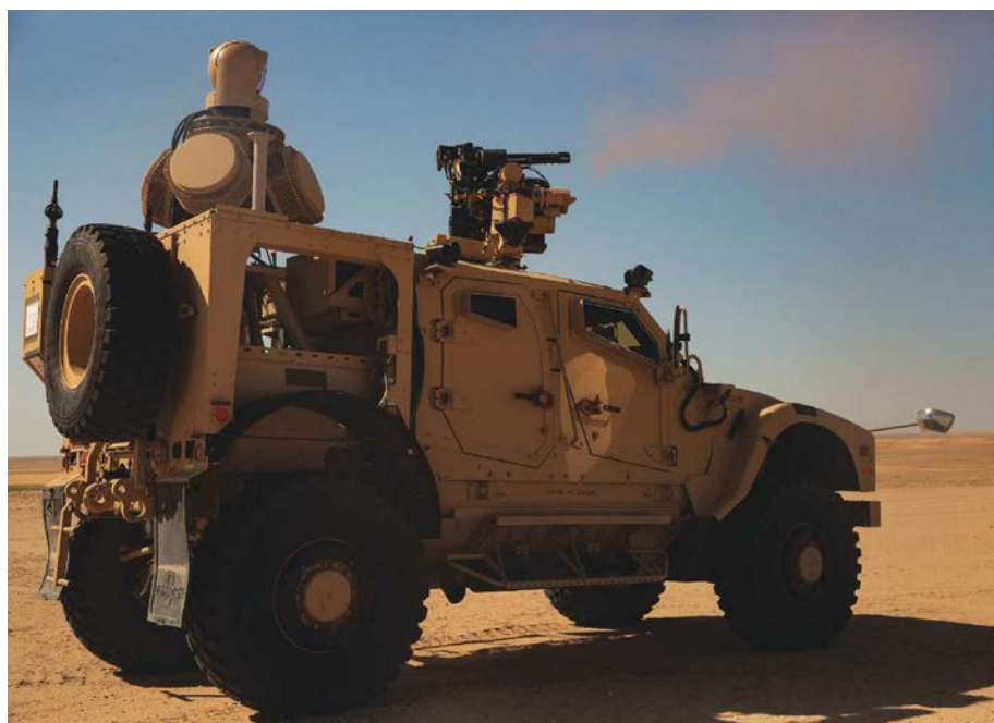
Above: A Mine Resistant Ambush Protected (MRAP) vehicle equipped with the MADIS was used by 2nd LAAD Bn during a live-fire range in Kuwait, Feb. 18. It is the first vehicle to utilize kinetic and non-kinetic measures to disable CUAS threats.
