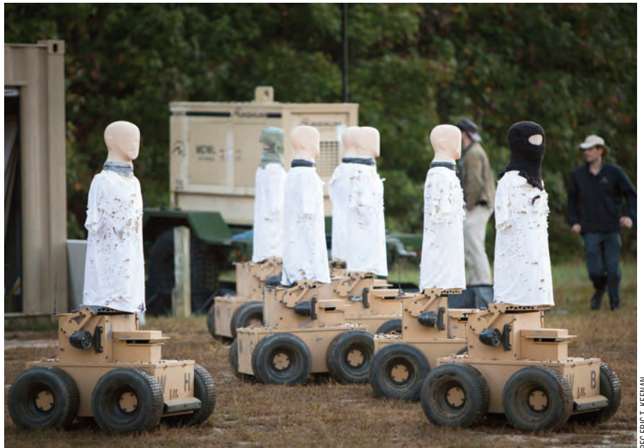
Above: Robotic moving targets were used throughout the LOE to depict life-size enemy combatants. The RMTs were developed by an Australian company, Marathon Targets, which assisted in the testing.
