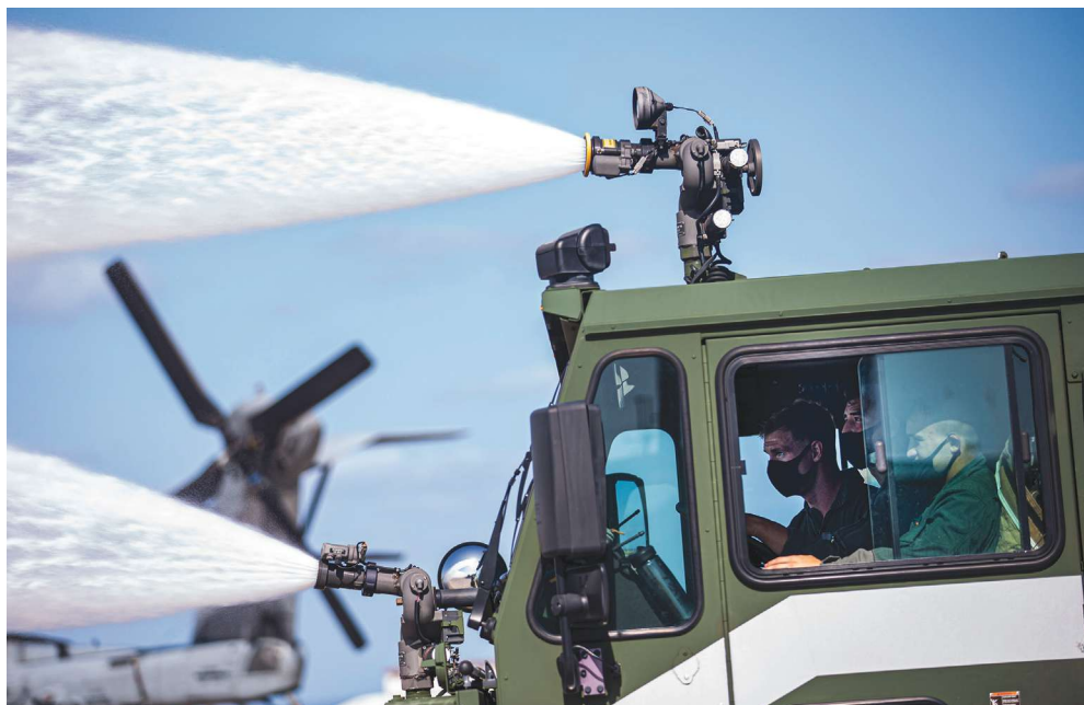
Marines with H&HS, MCIPAC conduct a turret drill with an Oshkosh P-19R Aircraft Rescue and Firefighting Vehicle on MCAS Futenma, Okinawa, Japan, April 7. EFR specialist Marines with H&HS provide aircraft rescue and firefighting services in support of airfield operations and respond to any fire-related emergencies and situations with a maximum response time of five minutes. (Photo by LCpl Alex Fairchild, USMC)
