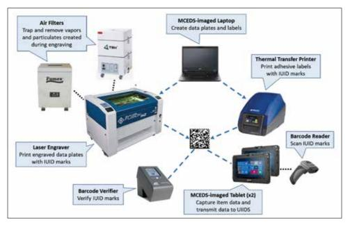
Figure 3. IMC components. (Figure provided by author.)
