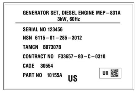
Figure 4. Marine Corps gold standard data plate. Example for military equipment (TAMCN items). (Figure provided by author.)
