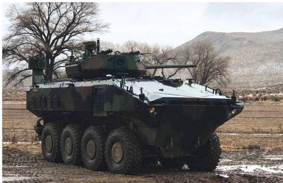
ACV-30 undergoing manufacturer testing incorporating the Kongsberg turret. (Photo by Kongsberg.)
