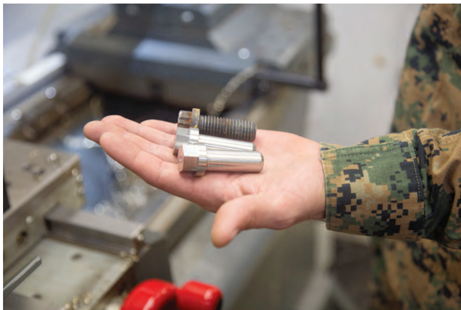
Additive manufacturing and 3D printing allow Marines to make replacement hardware at their duty station or while deployed. (Photo by LCpl Isabella Ortega.)
