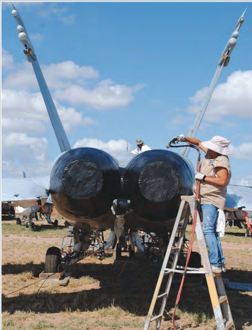
AMARG personnel spray a layer of black protective material onto an F/A-18 as they prepare it for storage, Sept. 9. The layers help lower the internal temperature of the aircraft, while also sealing up any crevices to keep dust, water and critters out.
