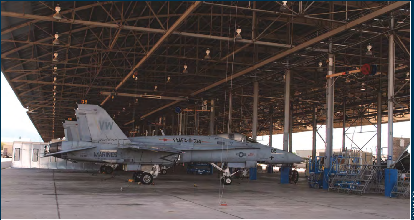
Above: A newly arrived USMC F/A-18 is temporarily stored under a shelter where technicians with the 309th AMARG will remove its egress system prior to the final stages of preservation, Sept. 9.
