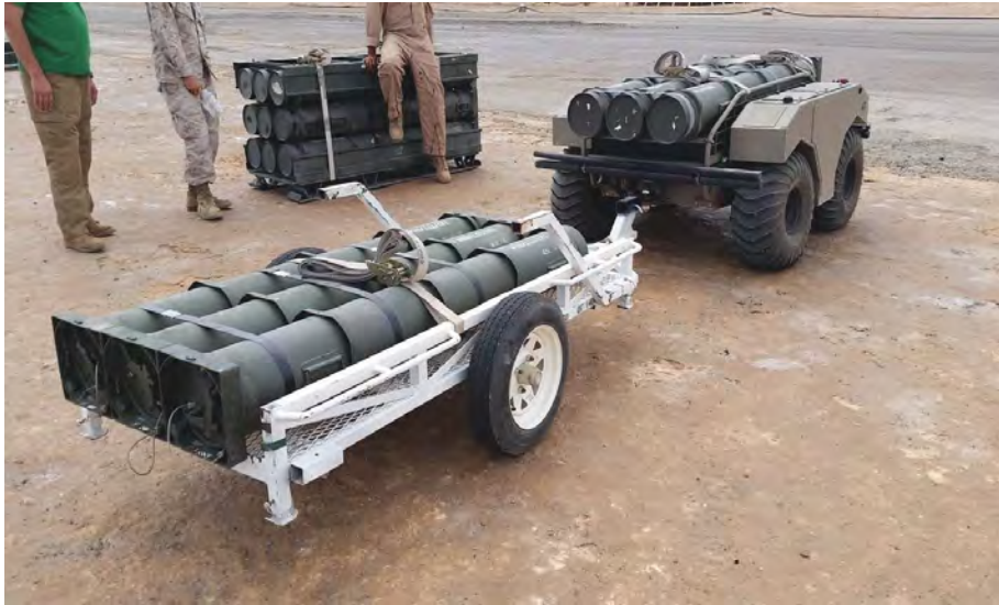
The SPOT with a load of rockets and towing a CART is a self-propelled ordnance transporter. (Photo provided by HQMC Aviation.)
