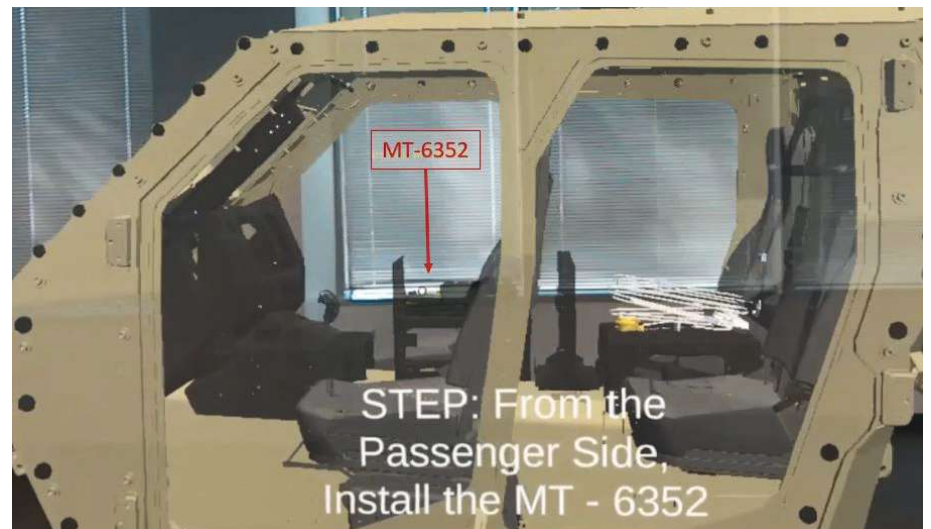
One step in the AR demo guide for installing a VRC radio using a JLTV model. (Photo by author.)
