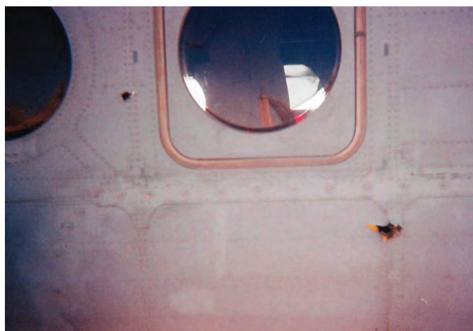
When the CO's war-torn Phrog was inspected, holes from at least 40 rounds were found in the aircraft. Note the bullet holes in the fuselage just above the ramp in the above left photo, and the holes along the side of the helicopter in the above right photo.
