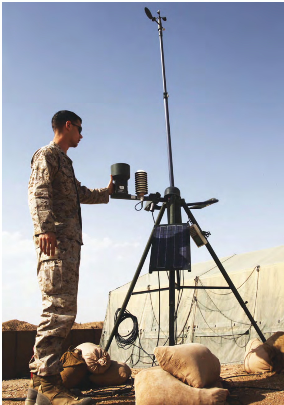
Sgt Zachary M. Salter checks the automated weather observation system at the Marine Air Control Squadron 2 compound at Camp Dwyer, Afghanistan, April 15, 2015. The system takes weather readings every five minutes and provides METOC analyst Marines with valuable atmospheric information.
