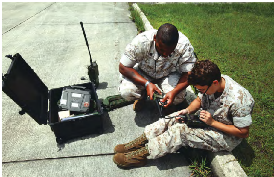
Sgt Brown and Cpl Cassie Mousaw operate the wideband tactical radio and the KILSWITCH tablets that allow aircraft crews to see specific information.
