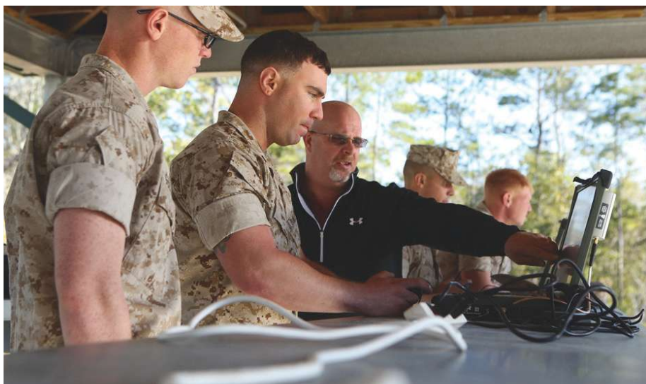
Marines with 2d CEB, 2dMarDiv learn to operate an R2C robot during a training exercise at MCB Camp Lejeune, N.C., March 11. R2C robots can scout for roadside bombs, search buildings and vehicles and are capable of traveling up to 800 meters from the control point.
