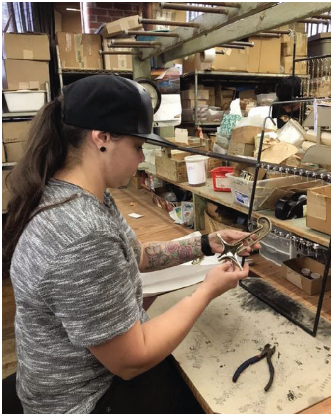
An employee at Ideal Plating prepares to string a sword hilt onto a rack to be replated. According to DeSenna, the prep work done prior to the actual plating is the most important step to ensuring the final product's finish is smooth and flawless.
