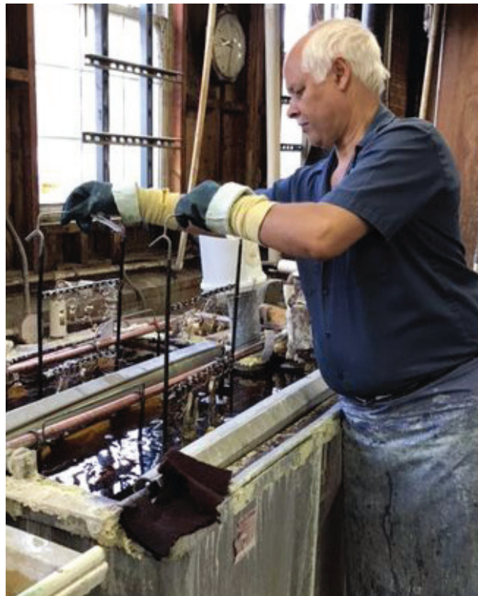
After the prep work is completed and the sword components have been strung, they are ready to be coated with nickel and plated in 24-karat gold.
