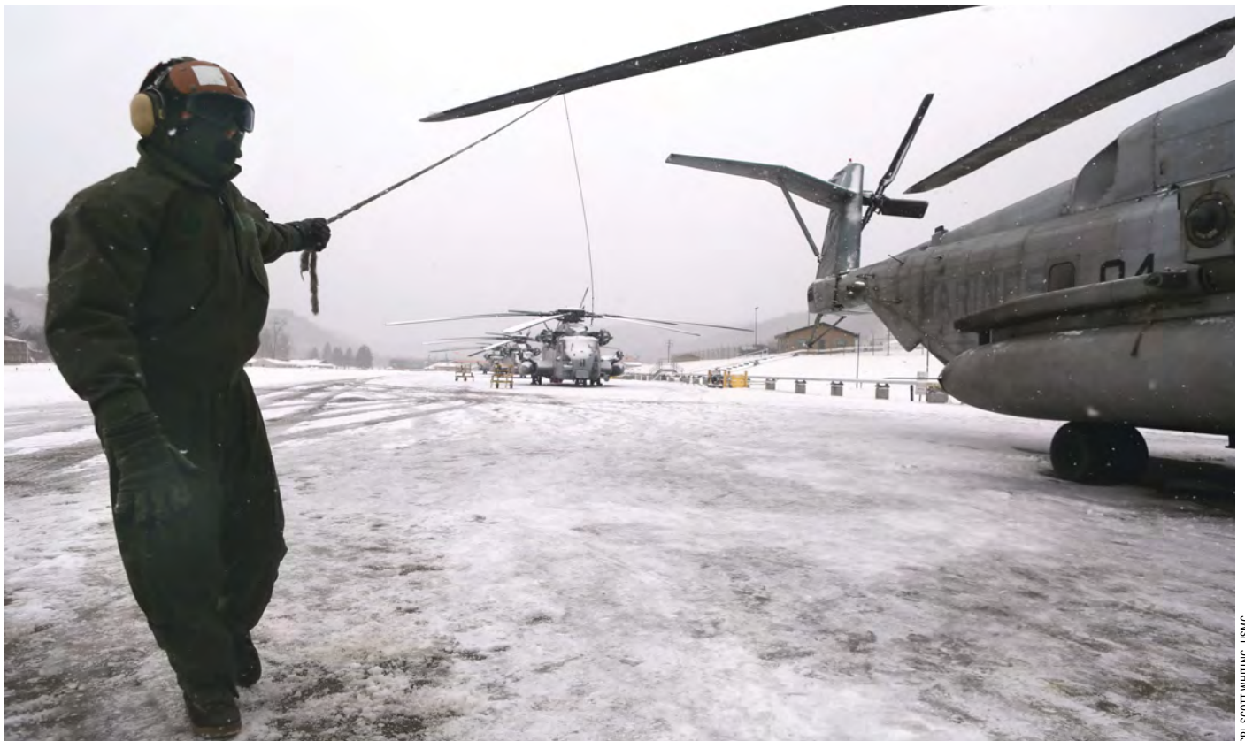
Cpl Adam Lindsey, a crew chief with HMH-464, manually rotates a propeller on a CH-53 Super Stallion to brush snow and ice off the blades during a DFT exercise at Camp Dawson, W.Va., in late January. Inclement weather required the Marines to take extra steps in preparing the helicopters for flight operations.
