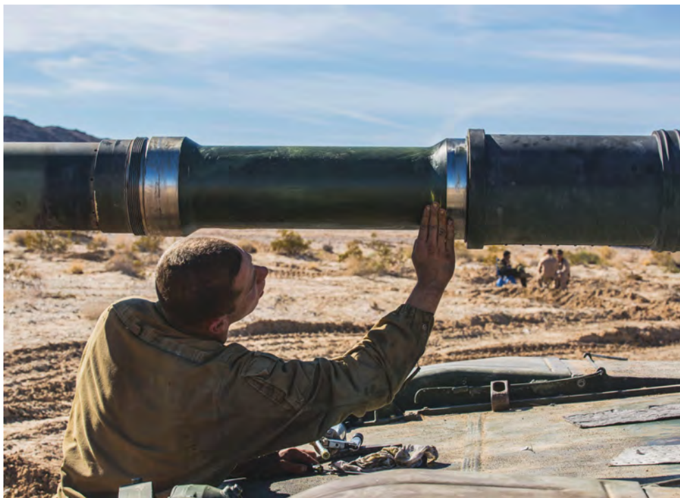
PFC Dylan F. McVey greases the bore evacuator on an M1A1 main battle tank in preparation for the TMAC during ITX 2-15 at MCAGCC Twentynine Palms, Calif., in early February. (Photo by LCpl William Hester, USMC)
