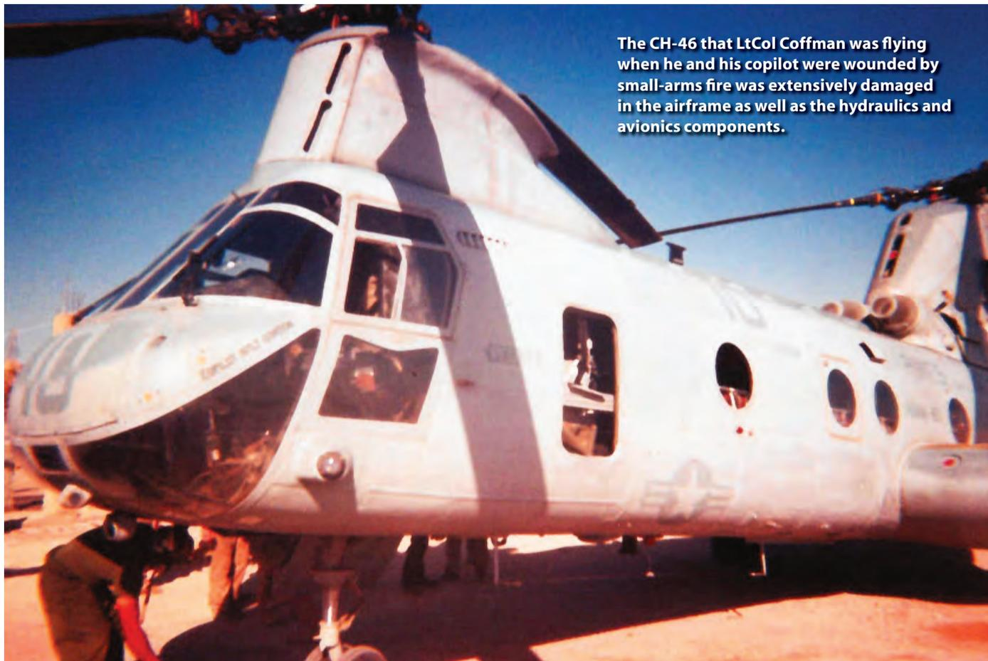
The CH-46 that LtCol Coffman was flying when he and his copilot were wounded by small-arms fire was extensively damaged in the airframe as well as the hydraulics and avionics components.
